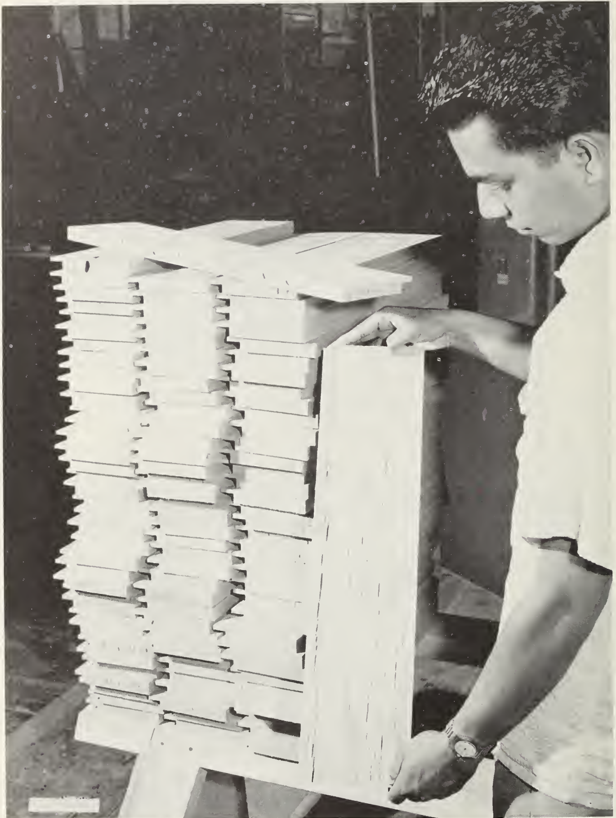
Figure 42. --Honeycomb checks in oak that show up when the boards are crosscut, ripped, or planed.
